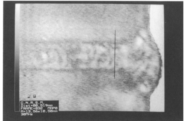
Fig. 2. Sample 1: acoustic micrograph taken at 30 MHz.
